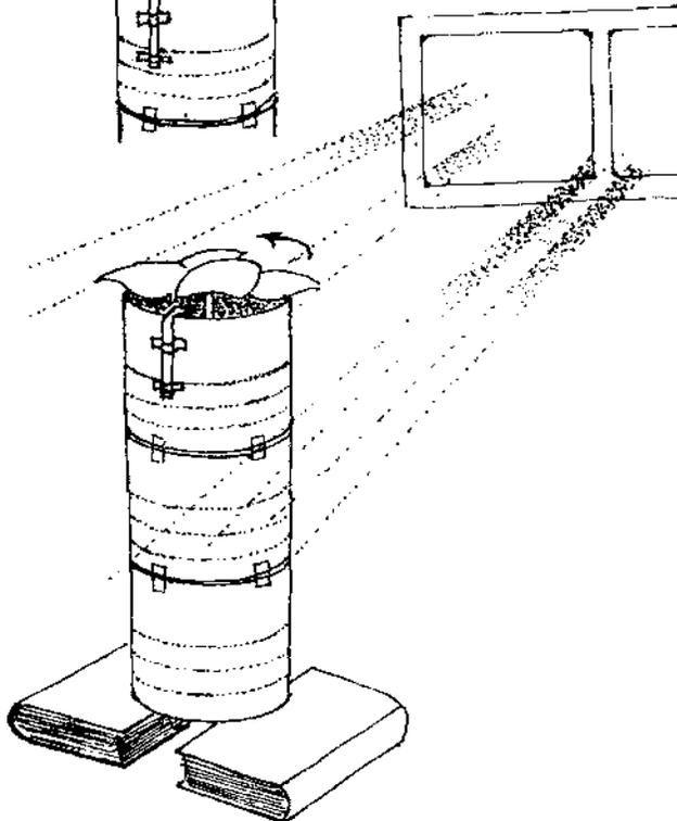
This simple device uses the sun's energy to rotate a pinwheel.
