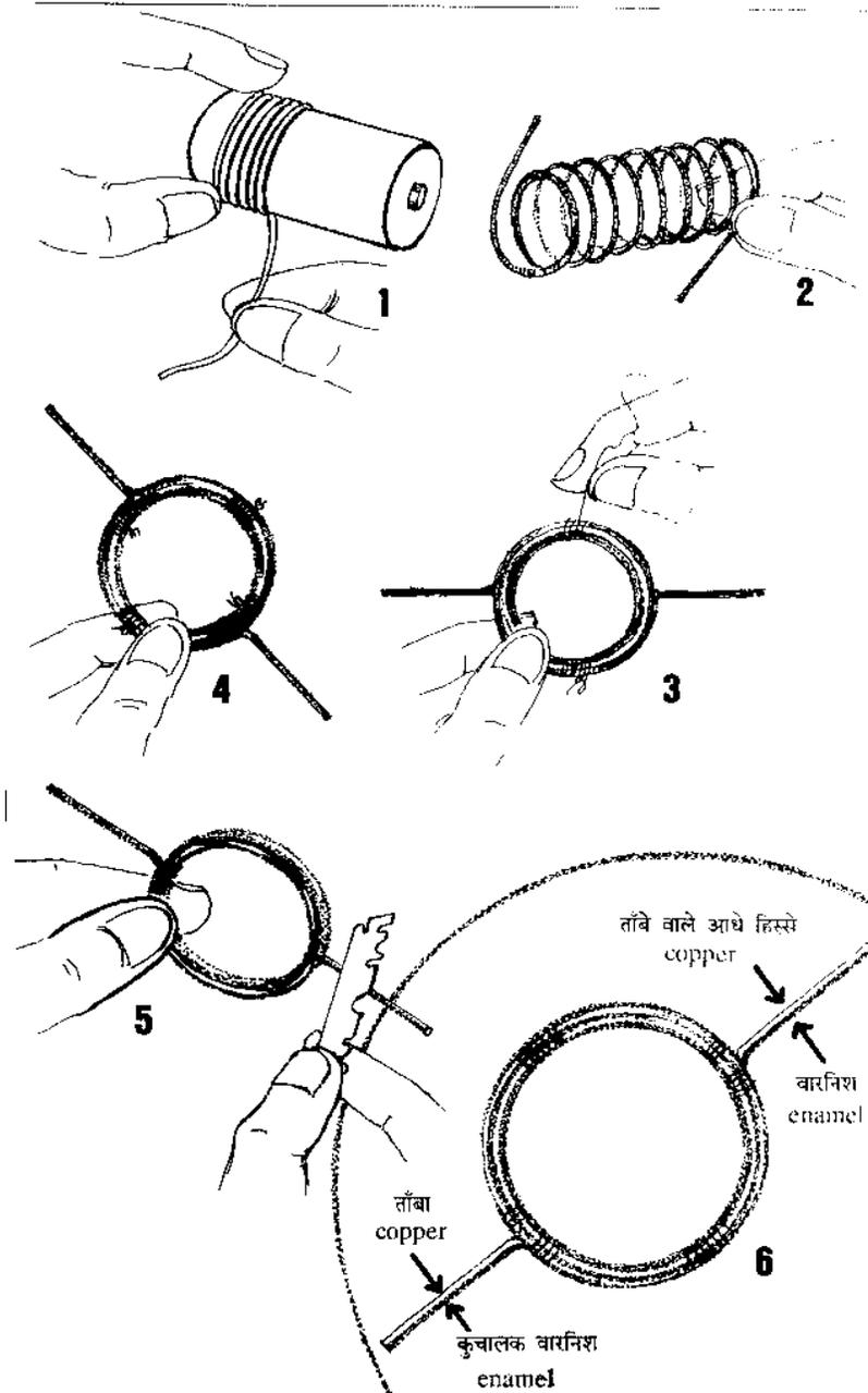
The copper/enamel sequence leads to make / break of the circuit and ensures that current flows in only half the rotation of the coil.
