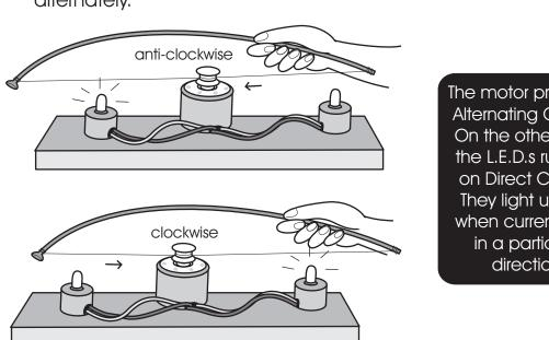
The motor produces Alternating Current. On the other hand the L.E.D.s run only on Direct Current. They light up only when current flows in a particular direction.
