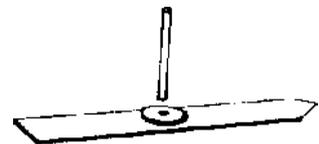
7. Cut a 15 cm long and 1 cm wide pointer out of cardboard. Stick another rubber disc at its centre. Insert an 8 cm long refill in this disc.
