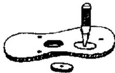
5. Punch a 2 mm hole in a 1 cm diameter rubber disc cut from an old slipper.
