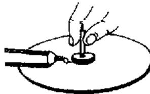
6. Stick this disc at the centre of a 15 cm diameter cardboard. Insert the 1 cm refill with the tip in this hole.
