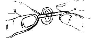
4. The refill goes in very smoothly. The refill on its own brass tip makes a very efficient bearing.
