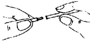
3. Insert the plastic refill in its brass tip.
